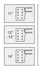
Hitch plate heights between 11" & 14" have the Clevis (U-shaped
