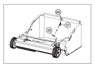
Thread Pull Handle (35) onto opposite end of the Pull Rope (37) as shown here:
