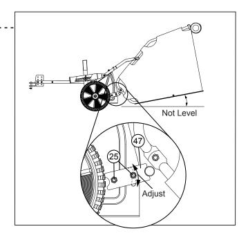
The sweeper Tow Tubes should be parallel with the ground (or angled slightly forward) when the sweeper is connected to the towing vehicle. If the Tow Tubes are angled rearward, adjust the Tow Tube mounting holes on the Clevis Assembly (68) lower. This will angle the Tow Tubes forward and raise the Hamper assembly.
