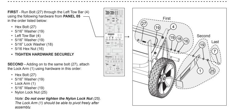
**LAST** - Slide the Vinyl Bolt Cap (7) over the end of the Bolt (27).
