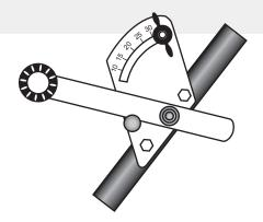
NOTE: When determining required setting, the edge of the wingnut is the marker, and not the center of wingnut. When the flow control handle is opened fully, the edge of the wingnut should be on the 30 mark.
