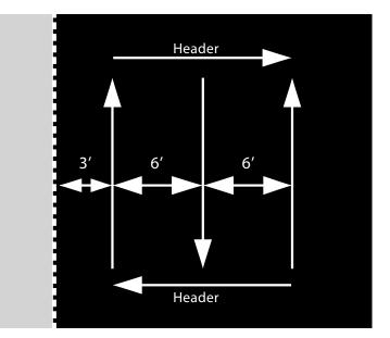
Additional spreading passes will be at the full spread width or approximately 6 ft. apart.
