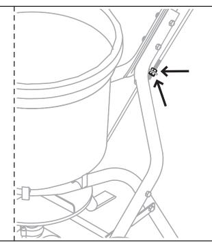
Hand tighten bottom nut on linkage rod until snug.
