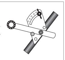
**IMPORTANT: REMEMBER TO START AND STOP** THE SPREAD WHILE MOVING. Do not open the flow control lever while stopped or material will simply run onto the ground without being spread.
