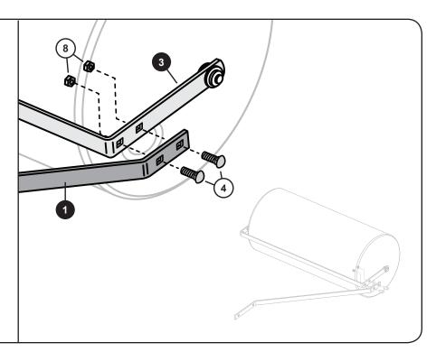
NOTE: Do not tighten the lock nuts added on this step completely (until Assembly Step 4-A is complete).
