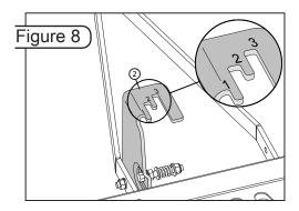
The Dethatcher has three possible Tine height settings on the Lift Lock (2) as shown in Figure 8.
