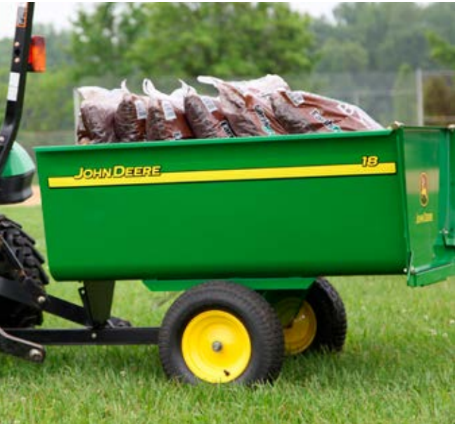
The John Deere Poly Carts feature a heavy-duty poly bed that won't dent or rust and are available in 650 lb. and 1000 lb. load capacities. Want to customize for special projects? The beds feature molded channels for adding dividers and side pockets for the addition of bed extensions as needed.
