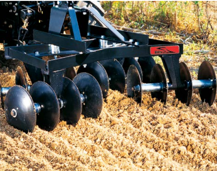
Use the Brinly Disc Harrow to break up rough, plowed ground effortlessly.
