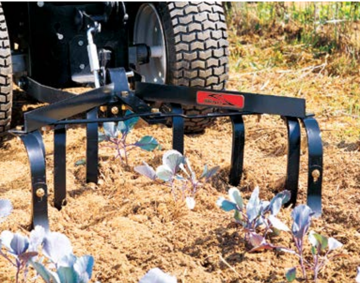
The Brinly Cultivator removes weeds and loosens soil between newly planted rows.
