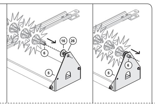
NOTE: Tines must not move from side to side inside opening of end panels.
