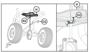
Slide the felt washer (N2) and fan (H) on the fan shaft.
