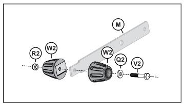
Assemble the gate lever handle  $(\mathbf{M})$  as illustrated using the following parts:
