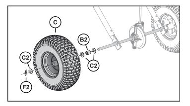
On the opposite end of the axle: Add a washer (C2), spacer (B2), another washer (C2), then the wheel (C).
