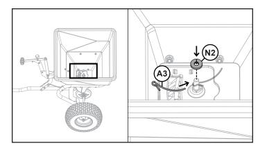
Slide the felt washer (N2) onto the fan shaft and insert the agitator pin (A3).
