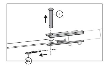
4. Hold spreader tow tube to remove pressure from hitch pin, then remove hitch pin (L) from hitch clevis and rear hitch plate or drawbar on machine.
