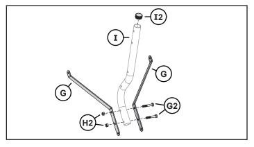
Insert the tube plug (**I2**) in the long end of the riser bar (**I**). Align the frame support brackets (**G**) with the riser bar (**I**) as illustrated. **LOOSELY** bolt these parts using:
