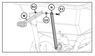
Place a Nylon Flange Bushing (U2) between the linkage arm (N) and gate lever (M). Bolt together using:
