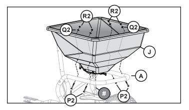
Place the hopper assembly (J) on top of the frame (A). Slide the fan shaft (#) through the bushing in the hopper bottom plate. Secure the hopper to the frame by using the following as illustrated above:
