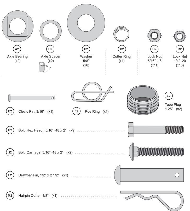
NOTE: An extra washer (C2) has been provided / may be remaining after assembly is complete.
