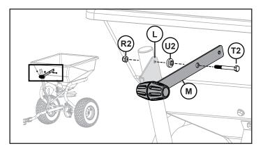
Align the gate lever (M) assembled in step 13-A with the stop bracket (L). Bolt **GENTLY** using the following parts:
