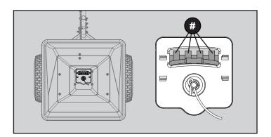
If spreading is long to the left of center, turn diffuser knob counterclockwise all the way; then turn knob clockwise until edge of diffuser plate (**#**) directs material slightly to outside of spreader as it falls on the spinner and test pattern is centered.
