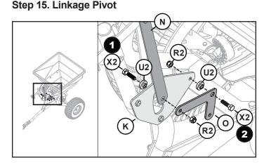
Attach linkage pivot (**O**) with hardware in the following order: NOTE: Bolt together snug but not tight.
