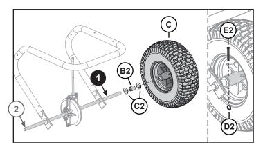
Note the location of the remaining axle holes. The wheel will need to be installed on the side marked "**1**" above.
