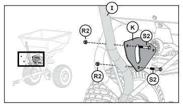
Align the pivot plate  $(\mathbf{K})$  to the riser bar  $(\mathbf{I})$  as illustrated. Secure with:
