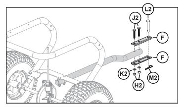
Align the clevis plates (**F**) with the towbar (**E**) as illustrated. Run two 5/16" x 2" carriage bolts (**J2**) through these parts and secure from below with two 5/16" washers (**K2**) and two 5/16" lock nuts (**H2**).
