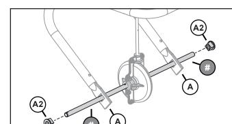
Add the bushings (**A2**) by sliding over the axle ends (#) and fitting in the square openings at the base of the frame (**A**).
