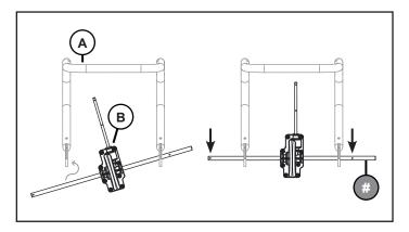
Alignment is crucial. The frame (A) and transmission (B) must be aligned as illustrated here.
