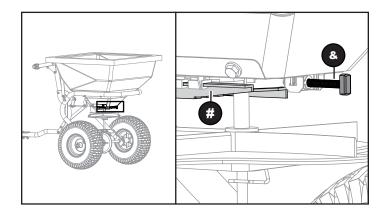
Adjusting knob (**&**) moves diffuser plate (**#**) forward and backward to center spread pattern and reduce side-throw (or skewing).
