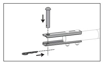
5. Pull or push spreader backward to disengage hitch clevis from machine hitch, install hitch pin in hitch clevis for storage and secure with 1/8 in. spring locking pin.
