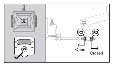
Adjust the position of the two lock nuts (R2) that were added on step 17-A such that the gate is in the no more that 1/16" past the fully closed position.
