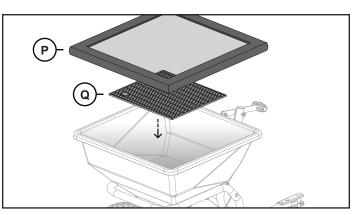
Place the screen (Q) down inside the hopper. Attach the hopper cover (P) by hooking it around the rim of the hopper.
