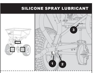
Apply the John Deere Aerosol Silicone Spray Lubricant to:
