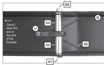
NOTE: Assemble the cart halves upside down on a flat surface. Use carton liners to support the cart halves.
