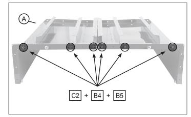
NOTE: When instructed, tighten until flat allen-head is flush with bed lip.
